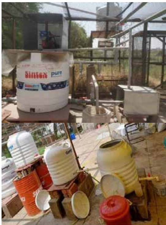
Cascade filter system for drip nutrification
